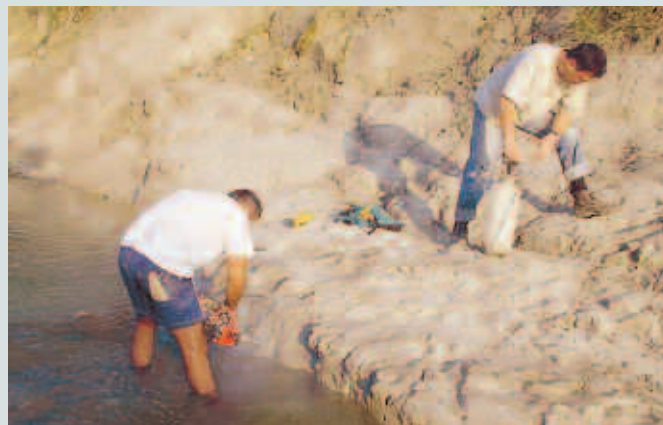
Our trusty drill, adapted from a chainsaw and still just as noisy, in action. Cooling water must be pumped through the diamond-tipped bit to prevent it overheating.
