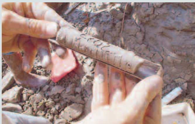
A typical core. The marks tell us the original orientation of our samples, vital if we want to tell the direction the magnets within were actually pointing.
