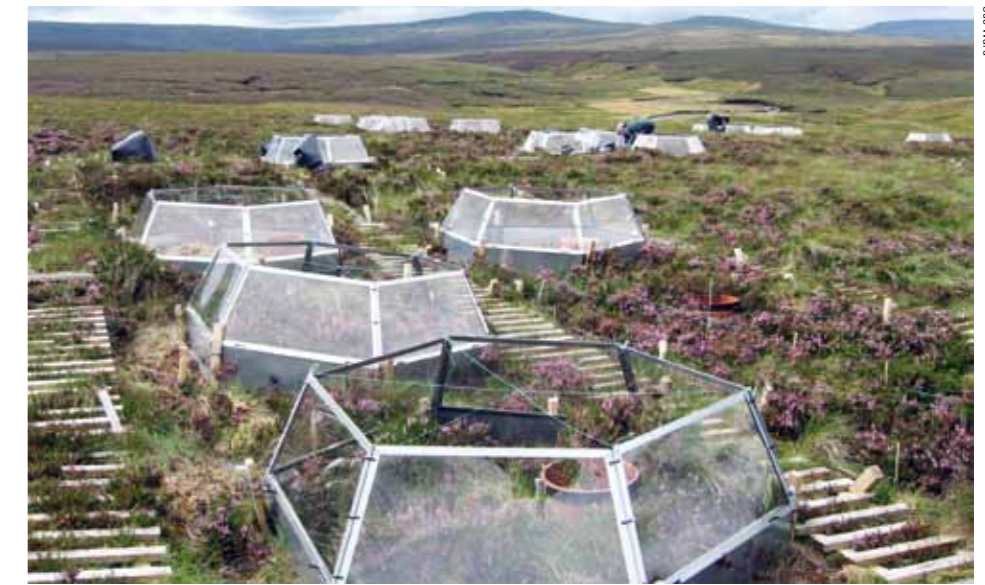
▲ The plant manipulation and warming experiment at Moor House National Nature Reserve, showing the passive warming chambers designed to increase temperatures by 1-2°C to mimic global warming.
