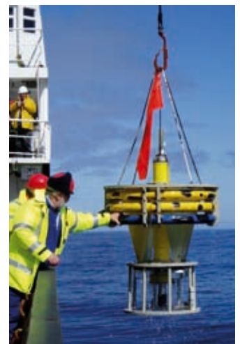
A drifting sediment trap collects samples of sinking material.
