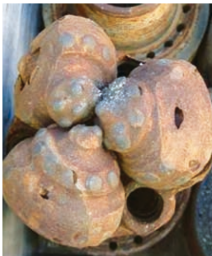
Damaged drill bit caused by drilling through granite and waters with high salinity.
