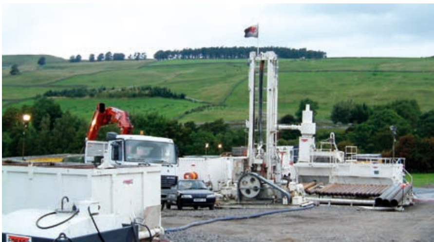
In search of cheap energy and new life. Drilling the 1000m Weardale borehole in Durham.
