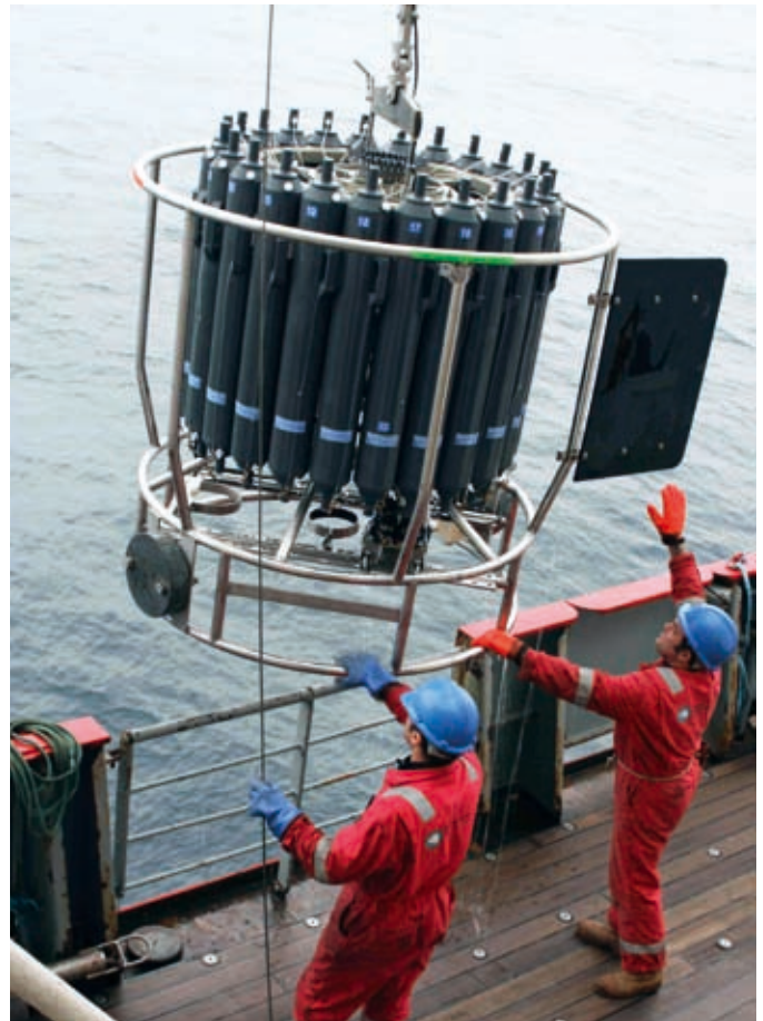
Water bottle rosette with 24 bottles at the side of the RRS James Clark Ross . The bottles are opened at pre-selected depths, as the rosette is lowered through the water, to take samples of the water near the gas bubbles.
