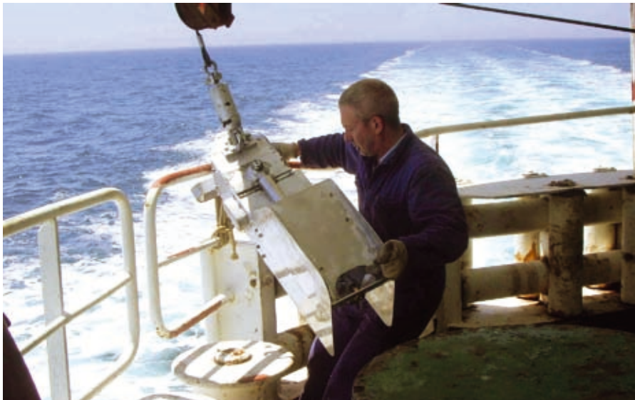
Launching the Continuous Plankton Recorder (CPR) from the back of the Pride of Bilbao .
