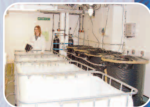
At PML we have developed the only lab in the UK for experiments with large quantities of seawater at predetermined and consistent pH.
