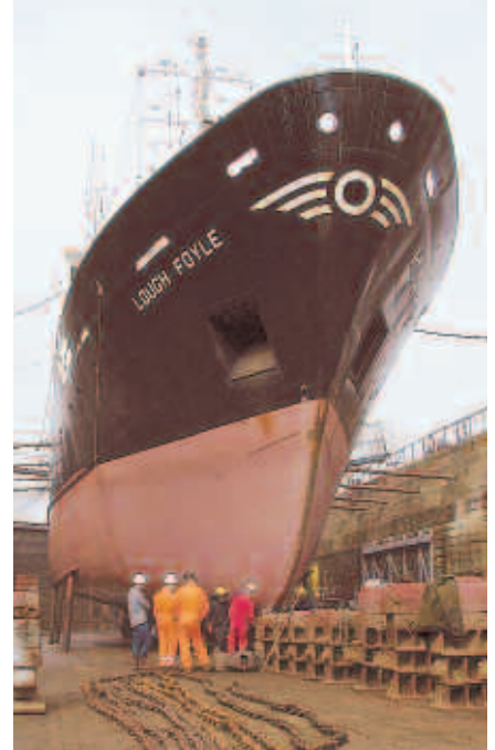
Engineers working to attach the multibeam transducer bracket to the Lough Foyle in the Garvel Dry Dock on the Clyde.
