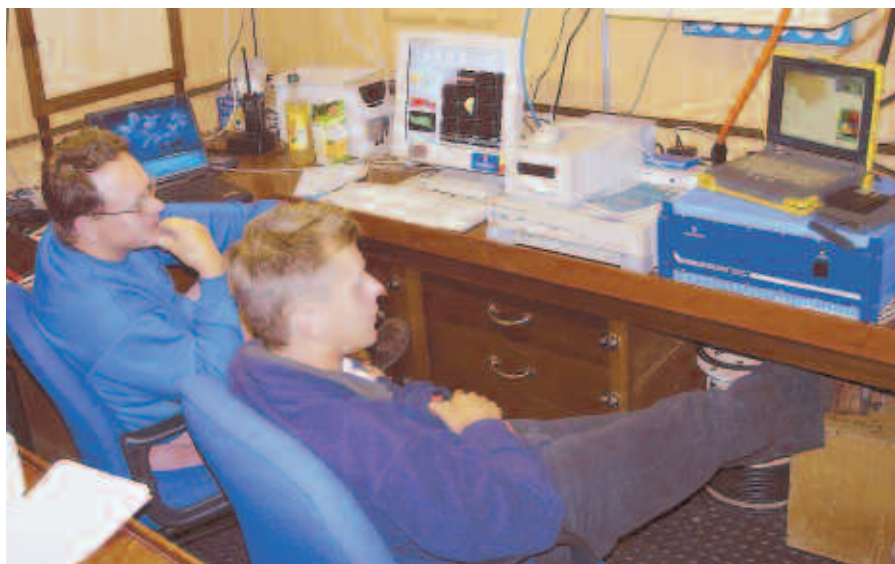
Sonar equipment controls and displays on board the Lough Foyle.
