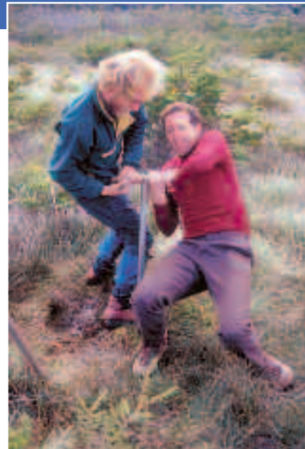
It's not always easy to sample the bottom of a bog! Bob McCulloch (left) and David Sugden (right) using a Russian corer to sample peat for radiocarbon dating. Strait of Magellan area, Patagonia, Chile.
